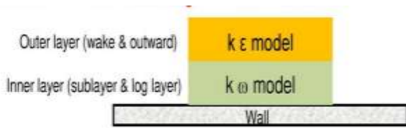
Figure 9: Visual representation of how SST combines k-ep and k-omega models
