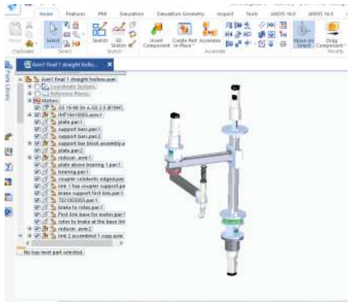
Fig-7: Assembly of SCARA ROBOT in Solid Edge
