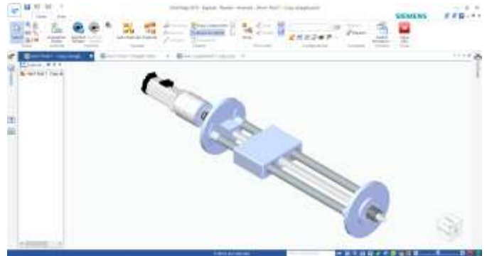
Fig-6: Design of vertical link in solid edge
