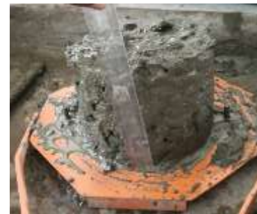
Fig-1: Slump cone test
