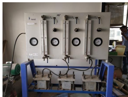
Fig.7, 8: Water Permeability Test
