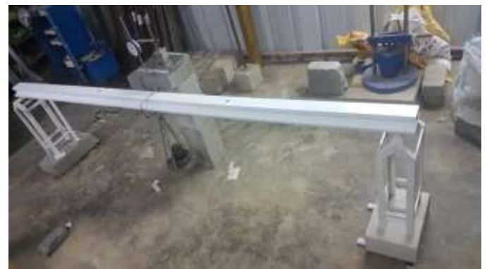
Fig -7: Deflection Test
