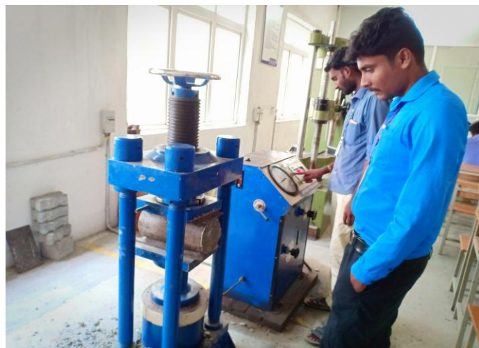
Fig -2: Split Tensile Strength Test
