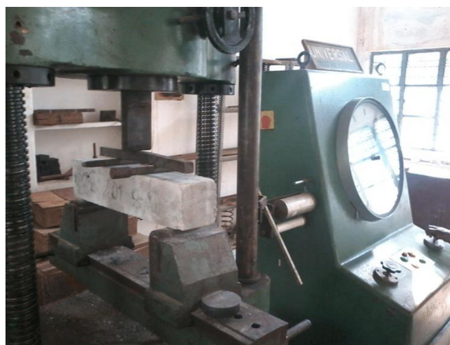
Fig 4 Testing of prism
