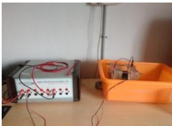
Fig 10 Setup for rapid chloride penetration test
