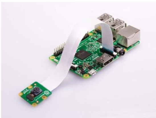
Fig: Raspberry pi camera diagram
