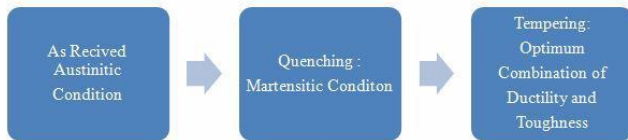
Fig.4 Sequence of heat treatment process of EN-24 Steel
