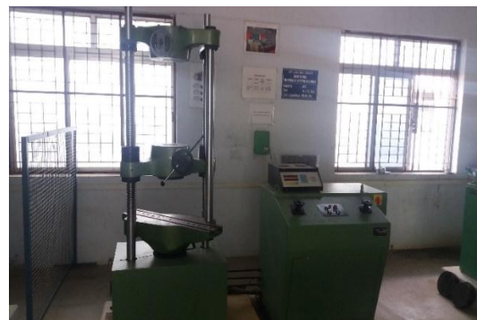
Fig.5 Tensile Loading UTM machine
