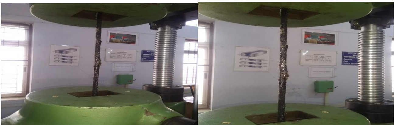
Fig.8 BFRP Retrofitted Elements Testing Under Tensile Loading
