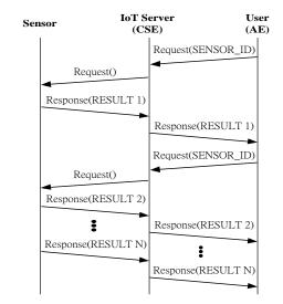
Fig - 3: The Passive scheme of D2ATC mechanism.
