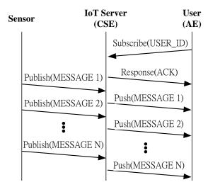
Fig - 2: The Active scheme of D<sup>2</sup>ATC mechanism.
