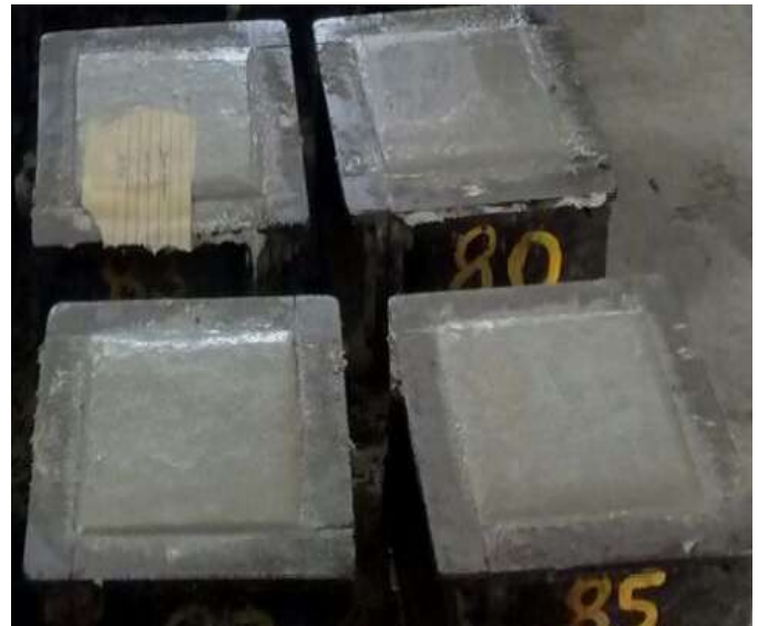
Fig. 2: Hardened concrete cubes inside the mould
