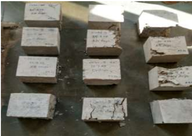
Fig. 6: Failed concrete cube samples after compression test
