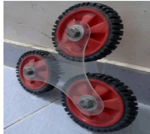
Figure 3: 3D view of wheel arrangement
