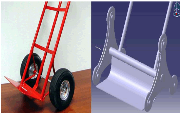
Figure 1: Initial design of Roller based wheel arrangement and wheel frame
