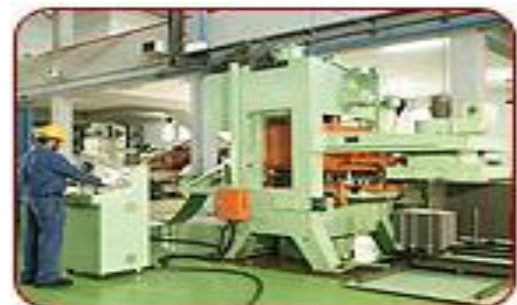
Fig 5: Aluminum Fin Generation Press
