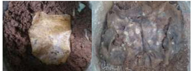
Fig -3: Banana film before and during biodegradation respectively
