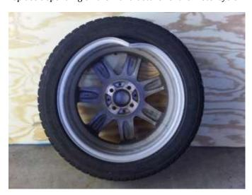
Fig -3: Bent rim of a car provided by "Rim Blades USA"
