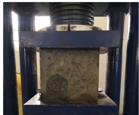
Fig -1: Compressive strength test on cube
