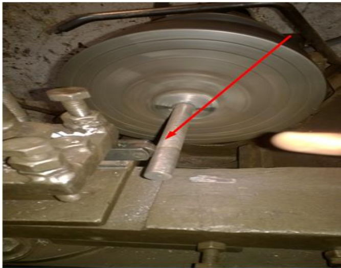
Fig-2.4: Performing Burnishing
