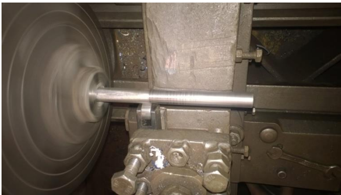
Fig-2.5: Performing Burnishing top view
