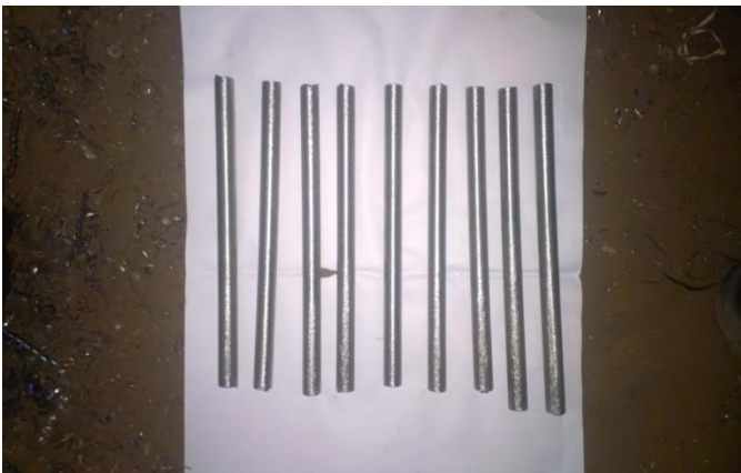
Fig-2: MS rod specimens before burnishing
