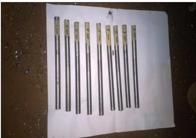
Fig-2.6: Specimens after Burnishing
