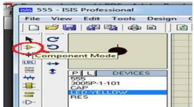
Select the all parts from library, that segments are added to devices list. Tap on the device and change the edge of the device by utilizing turn catches. At that point click in the work space then the chose segment is put in work space. Place every one of the devices in work space and put the cursor at the part stick end at that point draw the associations with that pen image. Interface every one of the segments as per circuit then that designed circuit is appear in below image.
