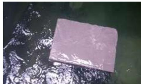
**Fig-1:** Floating of concrete cube
