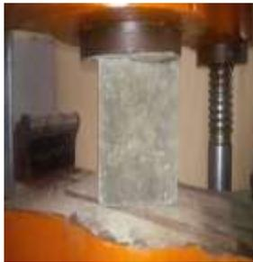
**Fig 2-** Compression Test on concrete cubes
