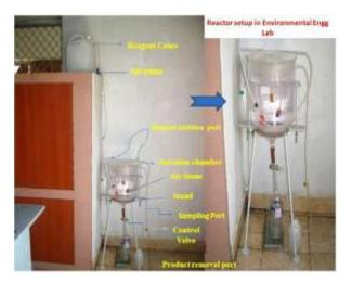
2. "Phosphorous Recovery through Struvite Crystallization: testing of parameters which enhance the recovery of Phosphorous"
