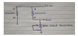
Fig 4:- Circuit Diagram of Alcohol Sensor
