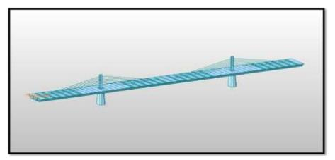
Fig-3: Iso view of the model showing different elements (cable, girder, pylon and pier)
