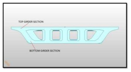
Fig-4: Girder cross-section of the model
