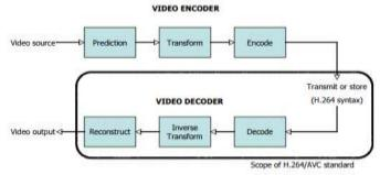
Fig. 1: Video Encoder and Video Decoder
