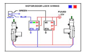
A door lock relay is a type of relay which consists of a mechanism which controls the door by sending power to the door lock actuators which helps in opening and closing the door.
