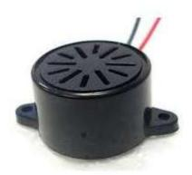
It is a device which is used to produce sound in case of an emergency. It consists of a small electromagnetic circuit consisting of a coil and a magnetic disk. When a current is passed through the coil, the coil produces fluctuating magnetic field due to which the disk vibrates at a frequency equal to that of an input drive signal.
