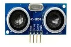
The Ultrasonic sensors emit short, high-frequency sound waves. These waves propagate in the air at the velocity of sound. If they hit an object, then they are reflected back as an echo signals to the sensor, which computes the distance on its own to the target, based on the time-interval between emitting the signal and receiving the echo.
