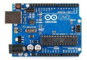
The Atmega 328 is a low-power CMOS 8-bit microcontroller which is based on a RISC architecture. It is powerful enough to execute instructions in a single clock cycle. It achieves the throughputs approaching 1MPS per MHZ allowing the system designed to optimize power consumption versus processing speed. Power saving is one of the important characteristics of it.
