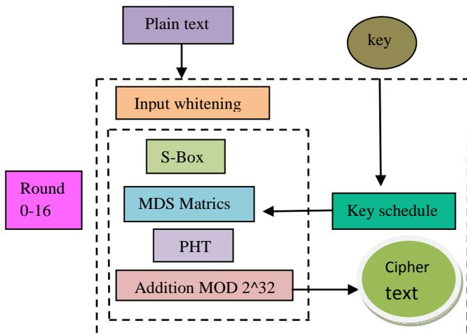
Figure 2: Process of Security Algorithm
