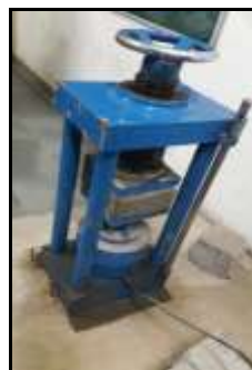
Figure-7 Testing of specimen at CTM
