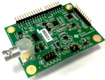
Fig-2: Vibration sensor
