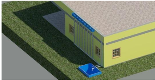
Fig -1: Collection of rainwater
