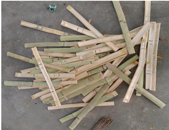
Fig -1: Bamboo splints chopped for reinforcement in beams
