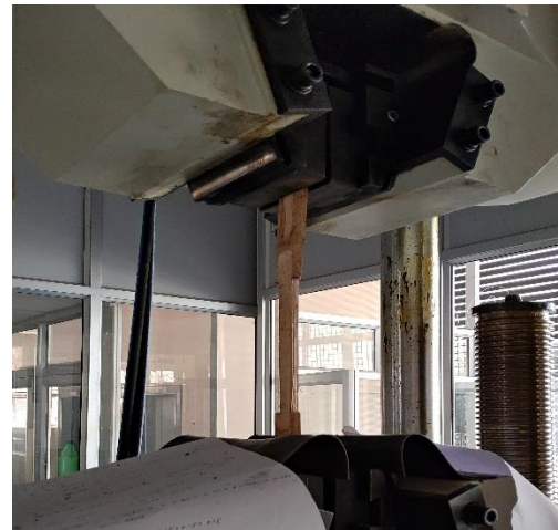
Fig-17: Tensile testing of bamboo splint subjected to alternate wetting and drying
