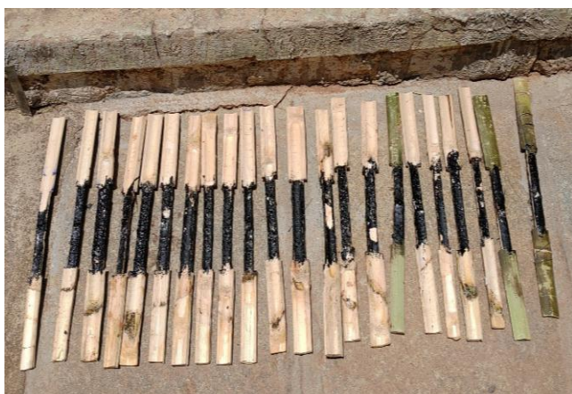
Fig-16: Bitumen coated bamboo splints drying in sunlight
