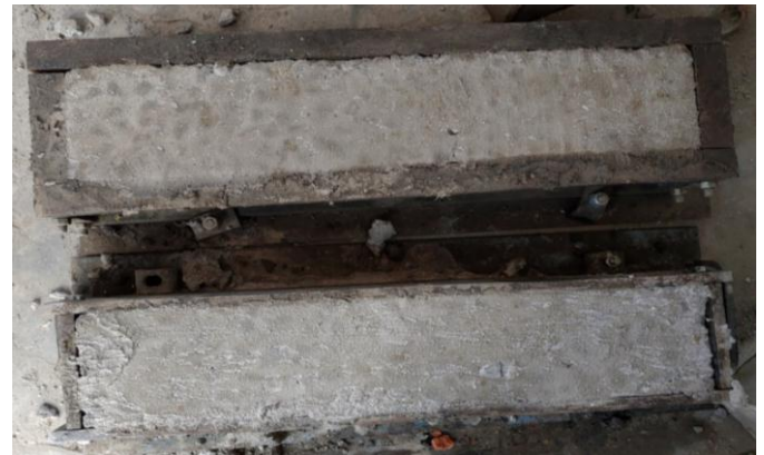
Fig-9: Hardened Beam specimens
