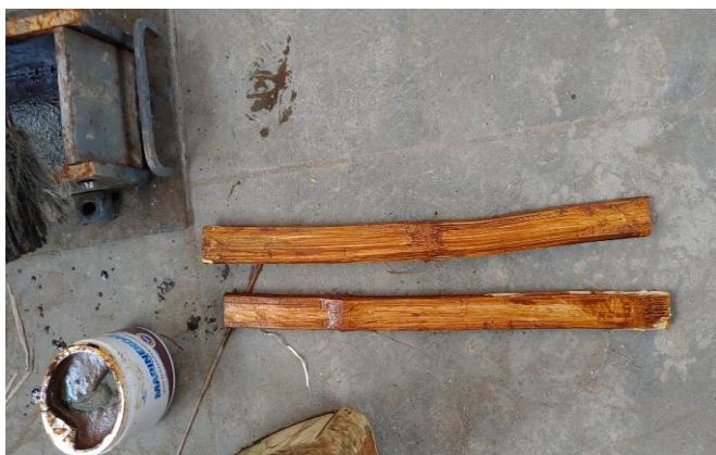
Fig-7: Polymer based Plywood coating being applied on splint
