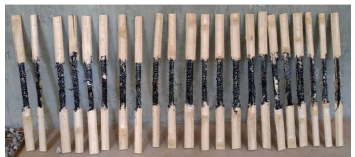
Fig-13: Bitumen coated bamboo splints
