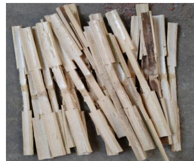
Fig-12: Bamboo splints ready for bitumen coating
