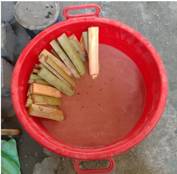
Fig-14: Bamboo splints dipped in solution
