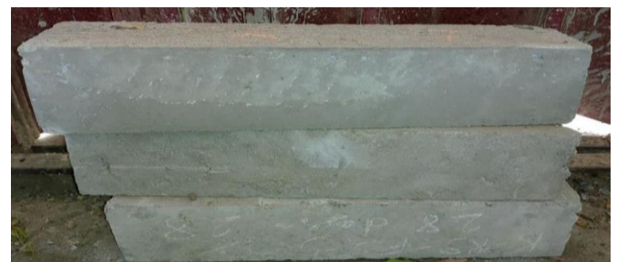
Fig-10: Hardened Beam specimens ready for testing
