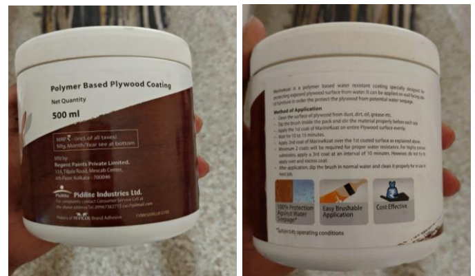
Fig-4: Pidilite plywood-based polymer coat as waterproofing for bamboo reinforcement
