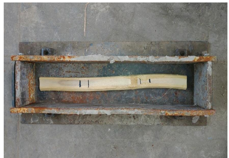
Fig-5: Placement of 1.25% of Uncoated Bamboo reinforcement in beam mould
