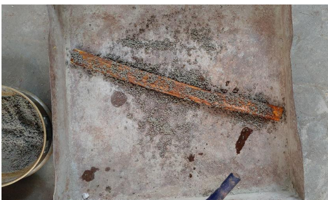
Fig-8: Coarse Sand sprinkled on top of Coated Bamboo Specimen
