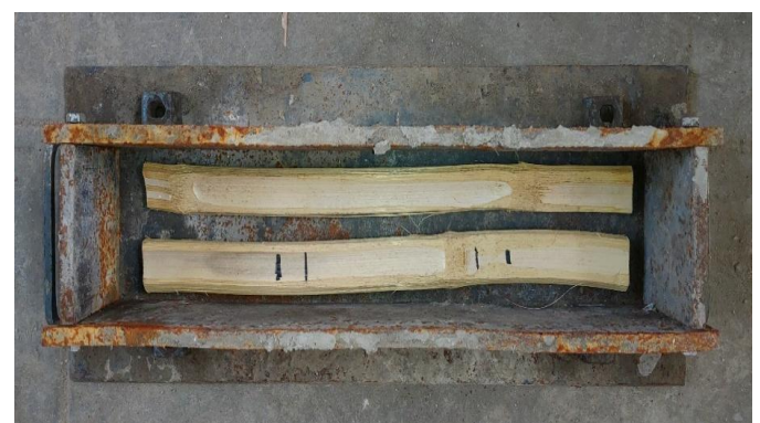
Fig-6: Placement of 1.25% of Uncoated Bamboo reinforcement in beam mould
