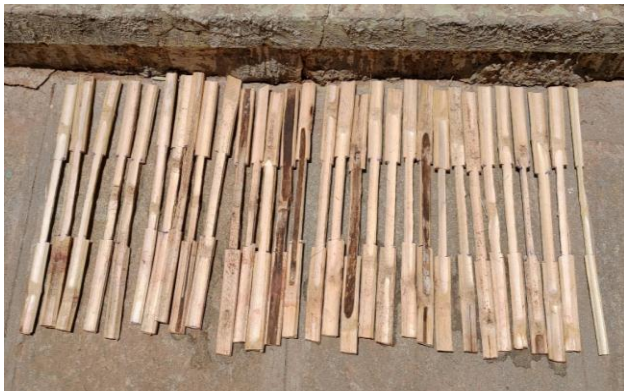
Fig-15: Uncoated bamboo splints drying in sunlight
