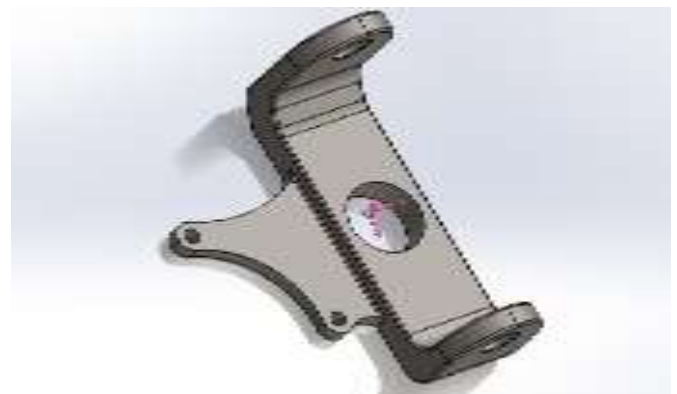
Fig -2: Knuckle Design in solid work
