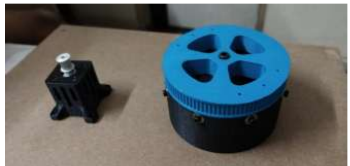
Fig.-4[2]: 3D printed gears of PLA created from this prototype.
