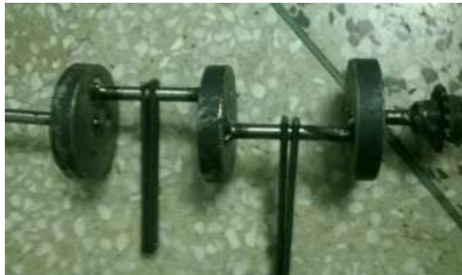
Fig.4. Final fabricated Crankshaft
