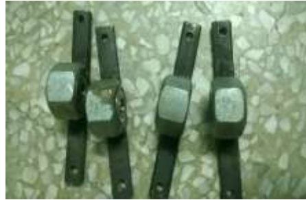
Fig.6. Final Welded Bearing to Metal Strip
