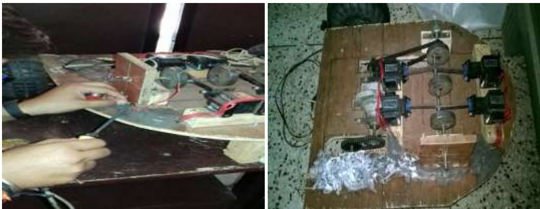
Fig.10. Final Setup of 4-Stroke Solenoid Engine
