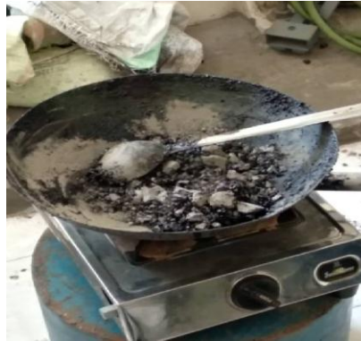
Fig 1: Mixing of Coated Aggregate and CRMB
