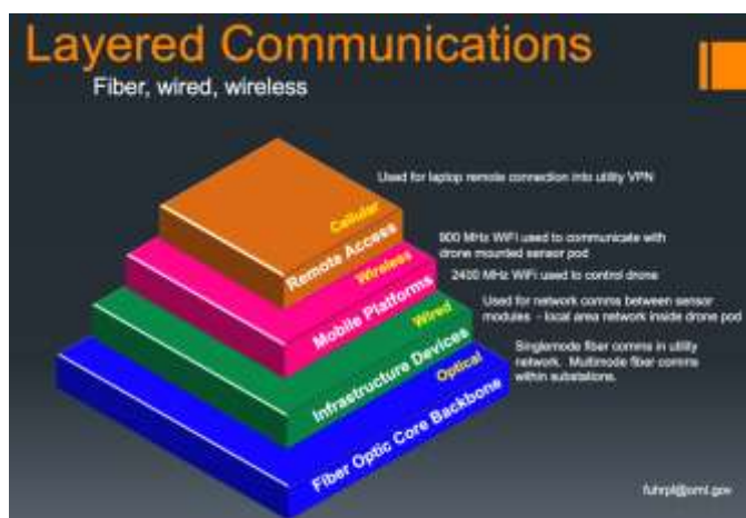
Fig. 2. Layered communications architecture for transport of signals and measurements from drone-mounted sensors to utility control center.
