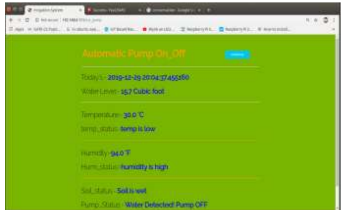
Fig- 14: Real-time Water_level Soil and Pump On_Off Status.
