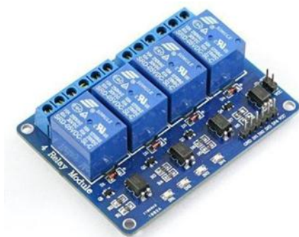
Fig -2: Relay board
