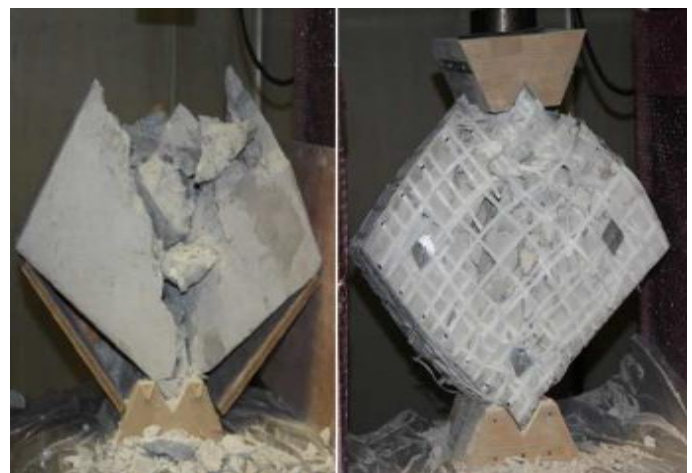
Fig -6: Non retrofitted specimen failure pattern and Retrofitted specimen failure pattern
