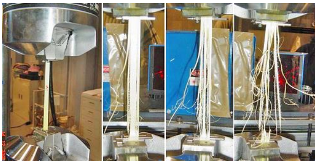
Fig. 3: Tensile test setup and failure pattern
