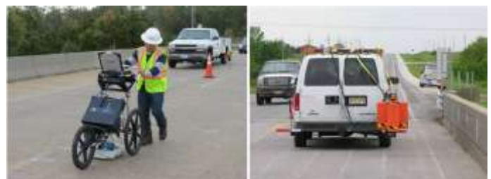
Figure 17: Ground-coupled GPR (left); Air-coupled GPR (right) [4]
