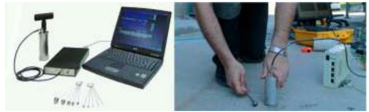
Figure 12: Impact-echo instruments (left) [49]; impact-echo testing on a slab [50]
