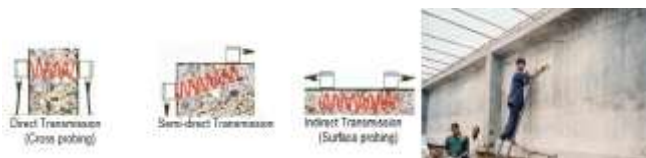
Figure 2: Different UPV methods and bridge girder testing by direct transmission method [15].
