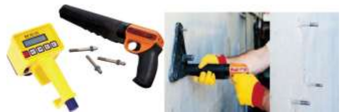
Figure 5: Windsor Probe instruments (left) [35]; equilateral triangle locating template used to positioning probes (middle) ; three probes at each corner (right) [36].
