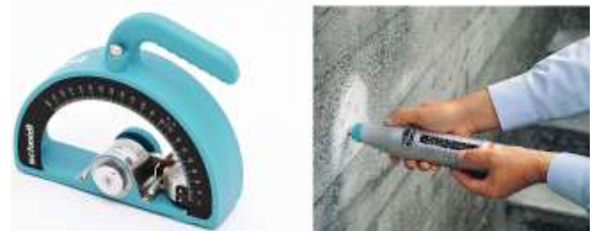
Figure 3: Schmidt OS-120 (left) [29]; Silver Schmidt hammer (right) [30]
