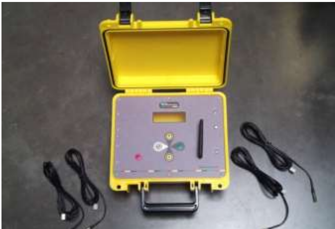
Figure 27: Maturity meter SensorConcrete [89]
