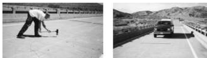
Figure 37: Model hammer excitation (left) and flatbed truck driving over a wood stud place on the center of the span (right) [123].
