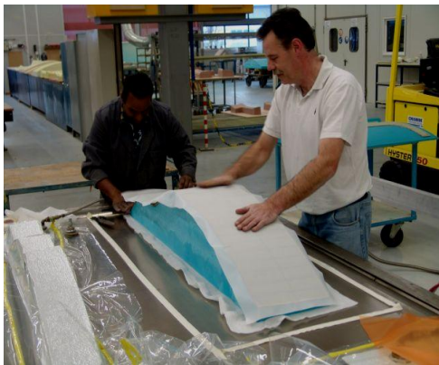
Fig. 2.2.1 vacuum bag molding preparations
