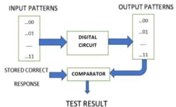
Fig1: Architecture of Test pattern
