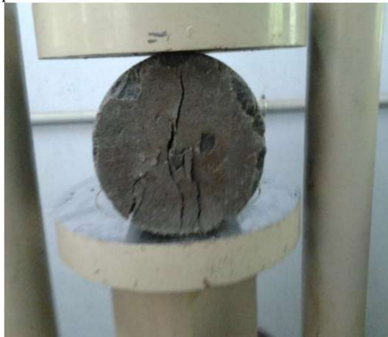
Fig. 4 Tensile testing machine with specimen[7]
