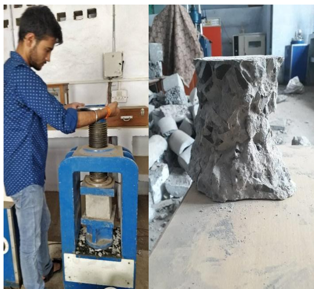
Figure 4.1: - Compressive Strength test and Breaking Cube
