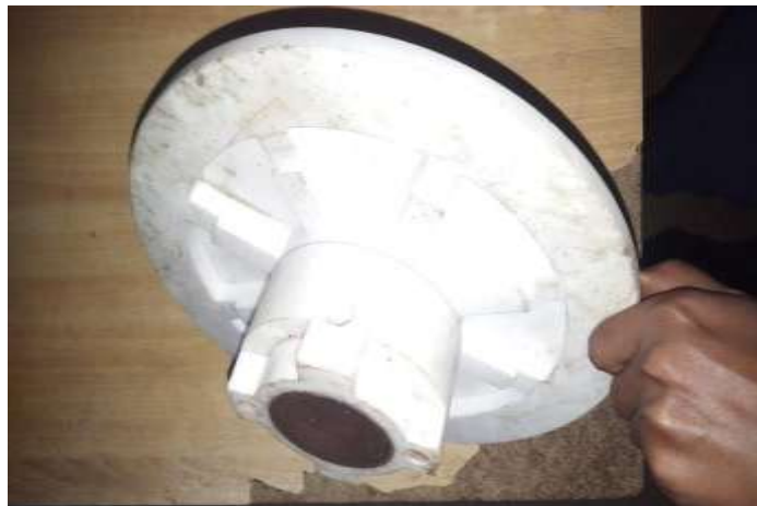
Fig -4: PP centrifugal pump stuffing box
