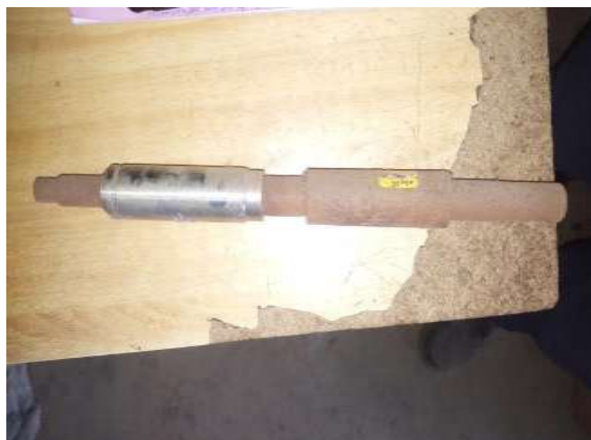
Fig -5: PP centrifugal pump EN8 shaft
