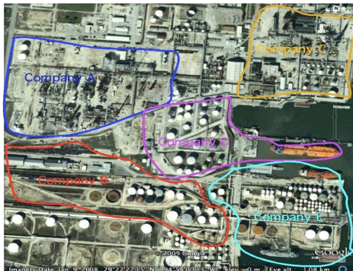
Fig. 7. Aerial view of the Texas (USA) ship channel where numerous industrial facilities are in close proximity to one another. Networks deployed at neighboring facilities will not “cross-talk” if non-routing nodes are deployed along the periphery of each facility.
