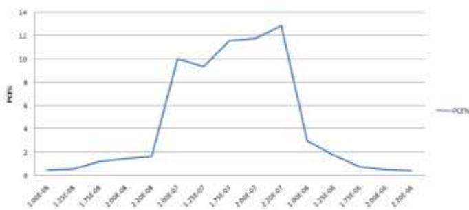
Fig 5. Effect of P3HT: PCBM layer thickness on PCE
