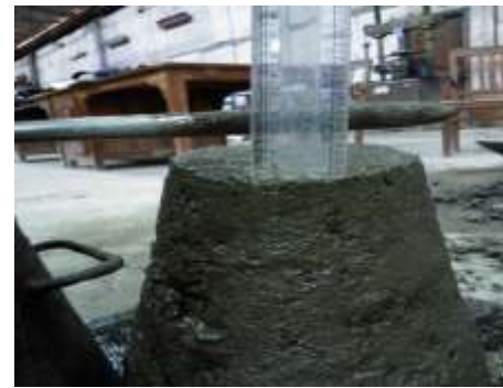
Fig-1: Slump Test
