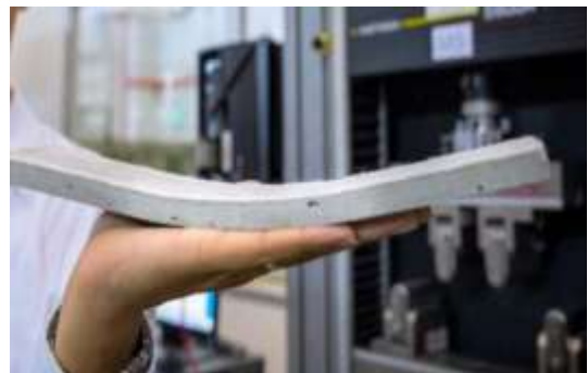
Fig -1: Behavior of ECC under flexural loading
