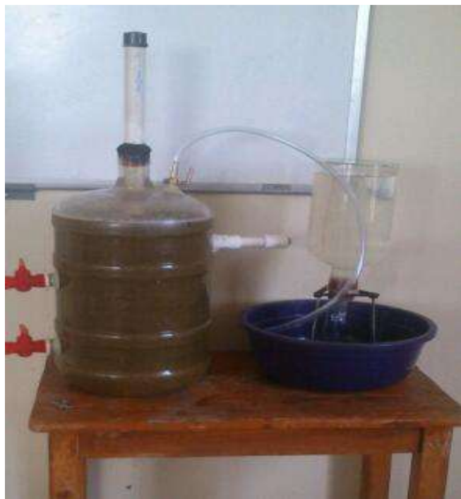
Figure: Anaerobic Digester
