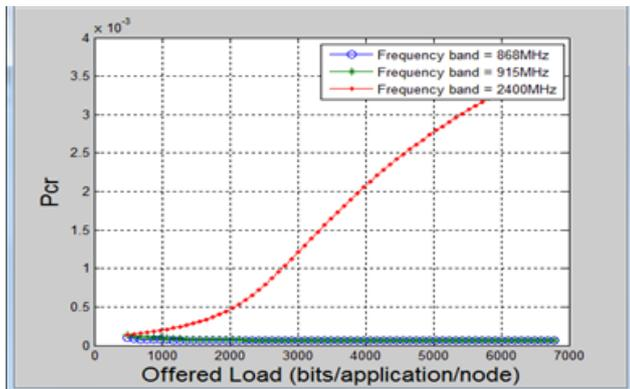
Fig 9: Failure transmission due to retry limits
