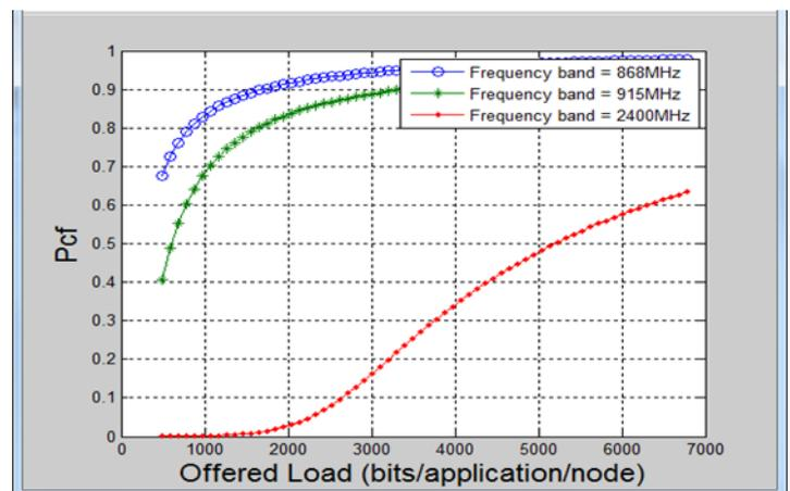
Fig. 7. Channel access Failure Probability
