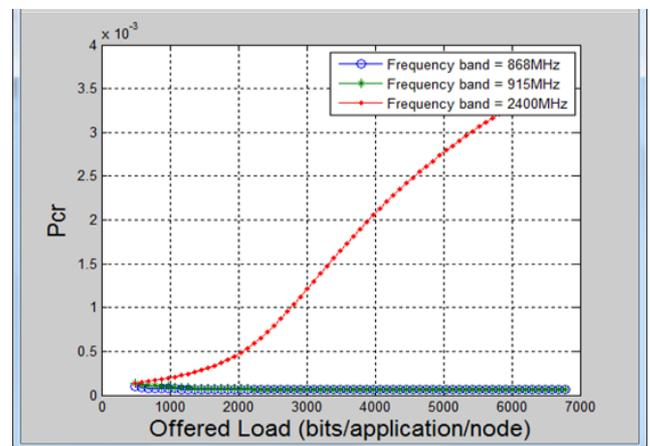
Fig. 8. Failure Transmission due to retry limits
