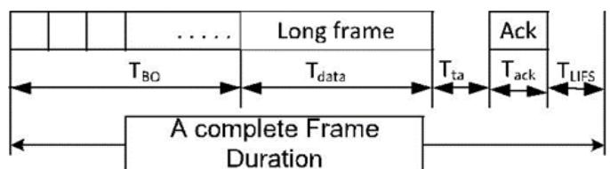
Fig. 3. Complete frame length including Acknowledgement and Inter frame Space
