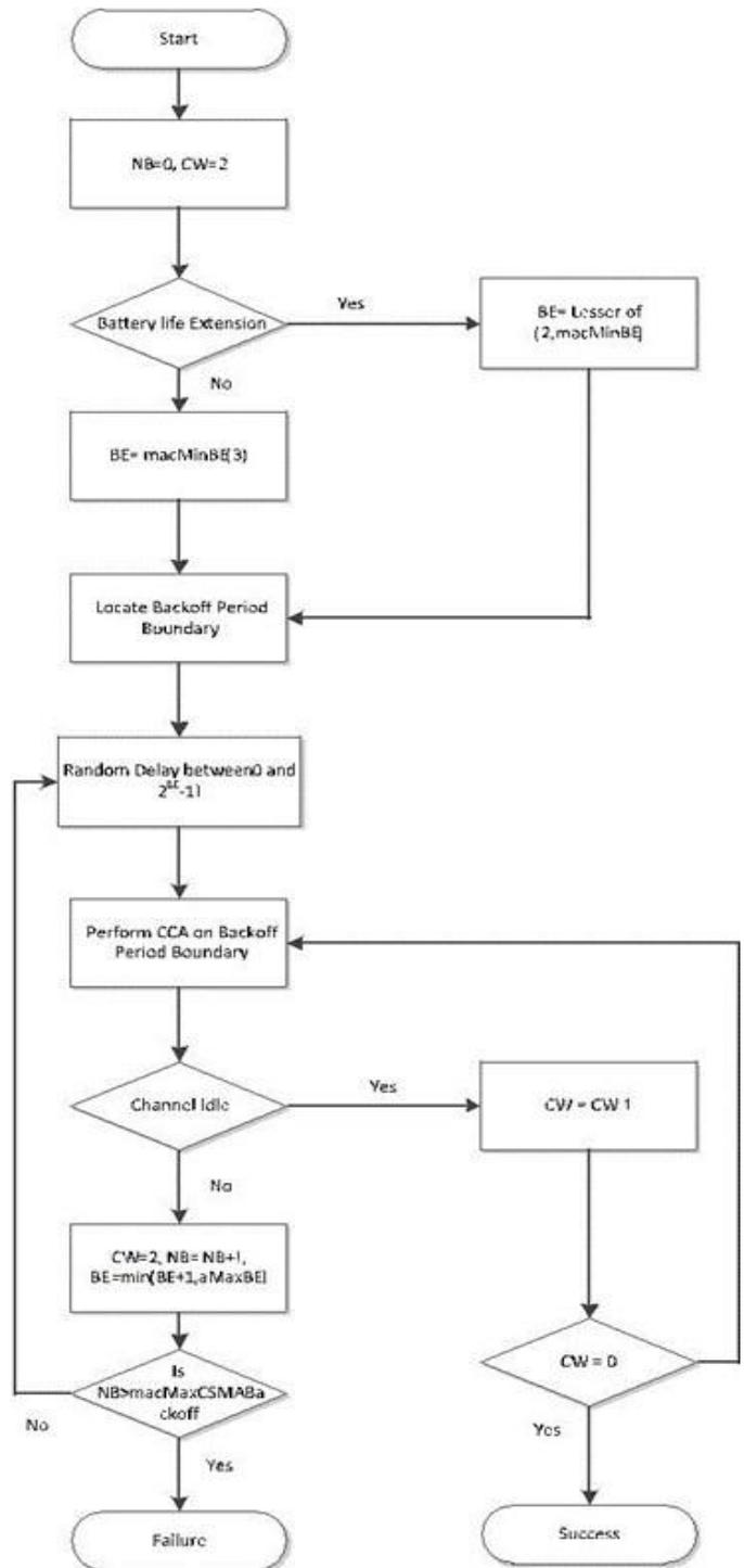
Fig. 2. Flow diagram of Slotted CSMA/CA
