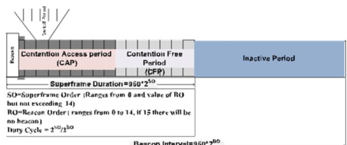
Fig. 1. Superframe Structure with CAP and CFP.
